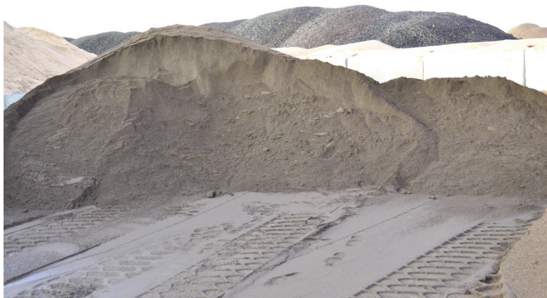
Stockpiles of pre-wetted lightweight aggregate, essential for internal curing of concrete, ready for use in high-performance construction projects.
