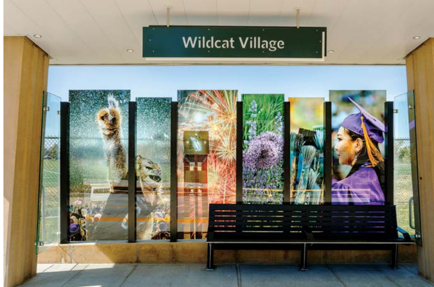
A laminated glass windscreen at the Wildcat Village station features We Are Weber , a photographic series capturing daily life and events at Weber State University. The imagery is digitally printed within glass, ensuring durability and long-term vibrancy.
