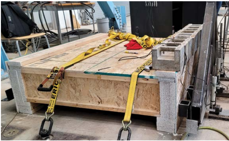
Typical specimen for shelf angles on 102 x 76 x 6.4 mm (3 x 3 x 0.25 in.) fiber-reinforced polymer (FRP) hollow structural sections (HSS) standoffs. PHOTO COURTESY SHIVAM SHARMA/UNIVERSITY OF WINDSOR
