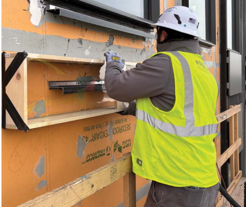
Chamber testing of repetitive cladding attachment components for air leakage in accordance with ASTM E1186 can verify the performance of typical fastener installations.
