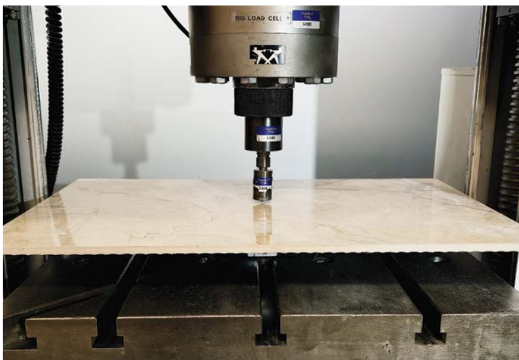
ANSI and ISO use completely different test methods of measuring breaking strength.
